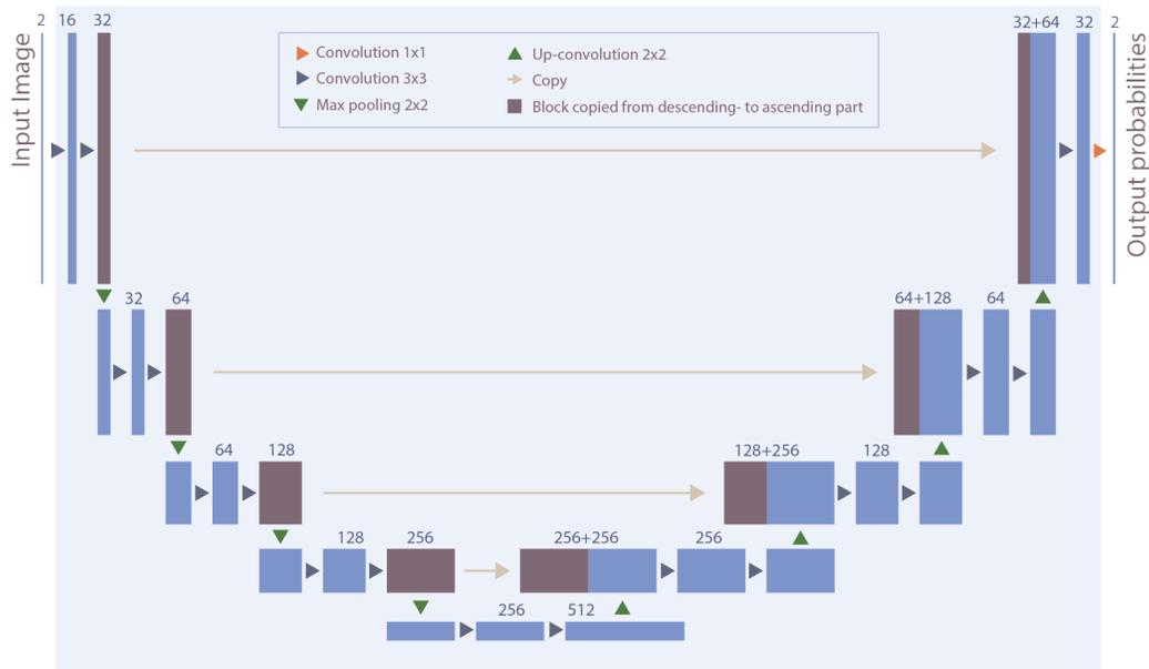
Figure 1: The fully convolutional network used for training our model. This is a U-net-like architecture<sup>16,17</sup> with slight modifications as described in the text.
